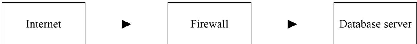
Firewall is a means of protecting servers and networks working online from unauthorized access.
